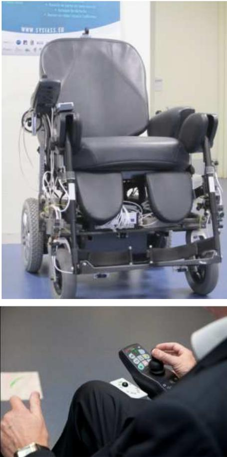
Figure 1: first prototype of the intelligent device for assisted navigation
