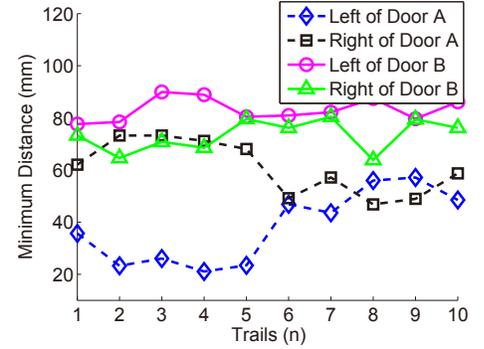
Fig. 7. Minimum distances of the robot to the edges of Door A and B.
