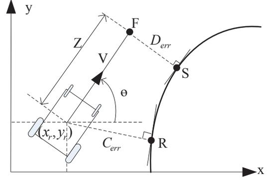
Fig. 4. The position error of the wheelchair [9].
